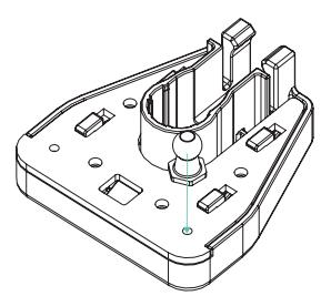
Install the metal pin under the shelf using the pre drilled holes. Attach the soft close support to the arm support (fig.1).
