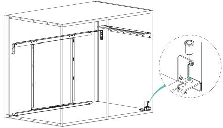
Fit the top pins of the side frame (C) into position in the lateral bracket (B) as shown (fig 1) Lower the bottom pin of the frame into the bush in the stop bracket (F) (Fig 3)
