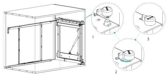
Slide the plain end of the centre pivot (I) into the guide at the bottom of the side frame (C) and fix in the position previously marked.
