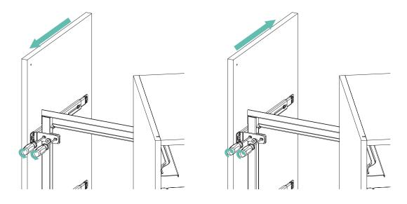
Tighten locking screws after adjustments are complete.
