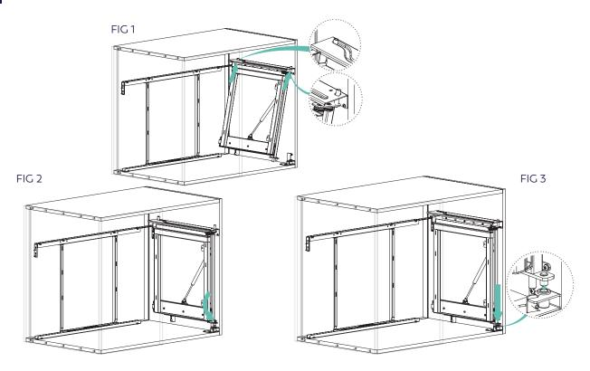
Fit the upper bushing (E) and turn until the tab locks into place.
