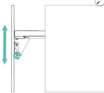
Adjust the door inclination to the front or to the back, then tighten the two M6x10 screws.
