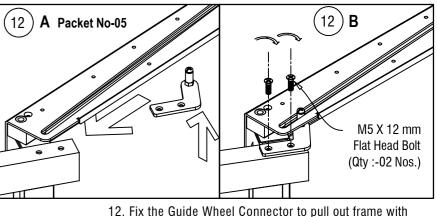
12. Fix the Guide Wheel Connector to pull out frame with 02 Nos M5 x 12 Flat Head bolts.
