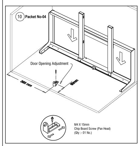
10. Fix the Door Opening Adjustment with One screw in the slot.
