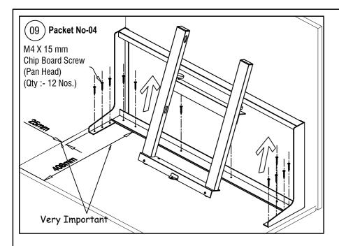
9. Fix the back frame as shown. Gap of 408 mm and 25 mm from edges is **very important**. Insert the back slide frame as shown.
